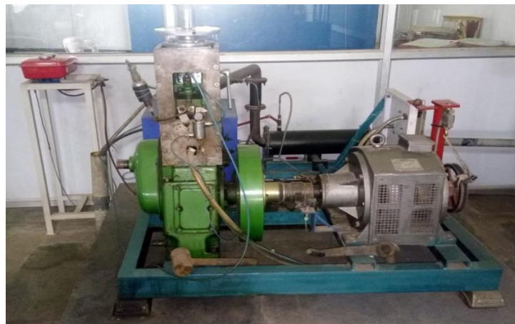
Fig.1: Experimental Setup (DI AV1 553DIESELENGINE)
