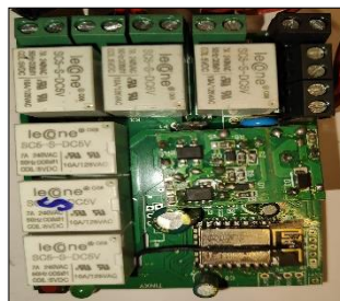
FIG 2: - It Is A 6 Node Smart Wifi Circuit, In Which We Can Run 6 Appliances, Such As Light, Fan, Ac, And Smart Appliances.
