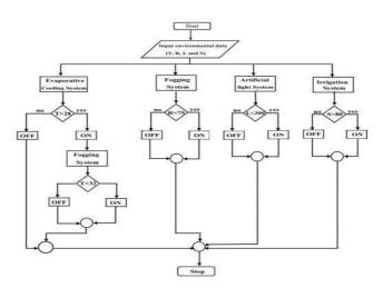
After connecting all the devices like Micro Controllers and Sensors, Irrigation systems control will be based on the data provided by the sensing devices. As shown in the control flow, some threshold value do exist for every control mechanism, until and unless the values are in safer boundaries, everything goes as planned. But if any abnormal values
