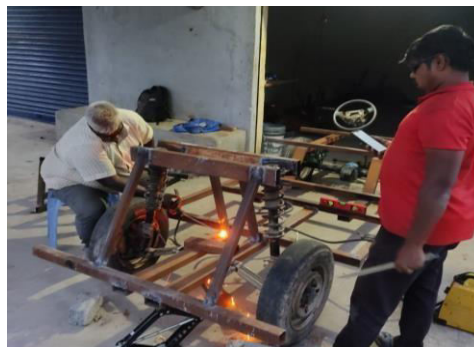
Figure 6 building the electric vehicle body
