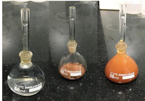
Figure 3.3 Specific gravity test by density bottle method.
