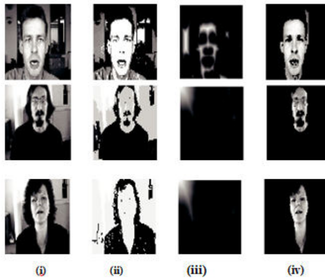
Figure. 2. (i) Original image (ii) Voronoi segmented image (iii) Segmented image after applying distance transformation (iv) Extracted face
