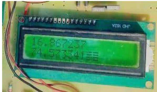
FIGURE 6 LCD Displaying Crack Detected Message STEP3 An alert message is provided to the concerned authorities together with the latitude and longitude values of the location where crack has been detected as shown in fig6
