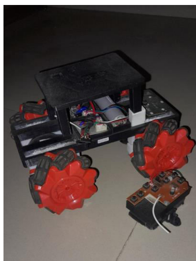
Fig. 2. Working model of 360 degree rotational vehicle.
