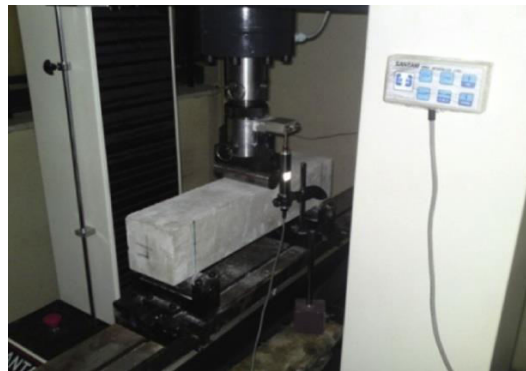
Fig. 4. Flexural strength test using “Universal Machine”.
