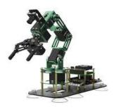
Dofbot is a compact, lightweight robotic arm designed for educational, research, and industrial applications. It offers precise control and is capable of performing tasks like pick-and-place, assembly, and 3D printing. Dofbot is often used to teach robotics and automation, with features like easy programmability, high precision, and flexibility for various applications.
