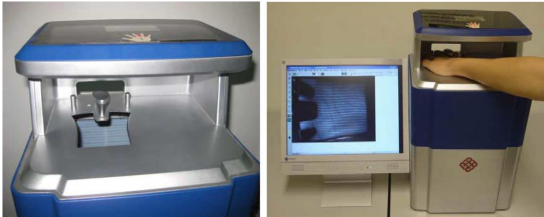
Fig. 1. Developed palm print authentication system with structured light imaging and an example of the use of the system.
