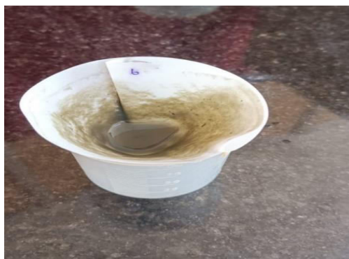
Fig.3 effluent extraction on a filter paper
