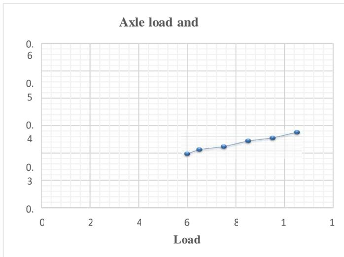
Graph Showing the relation between Load class and Stress ratio for single loaded axle
