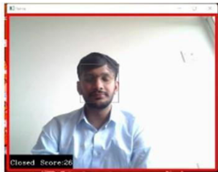
Figure 3: Show the real time test case generating a score based on the time the eyes were closed and sounding an alarm when reaching certain threshold.
