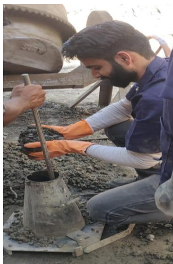
Figure 2 Slump Cone Test
