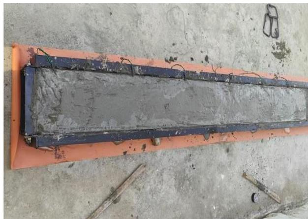
Fig 1:Casting Of Specimen
