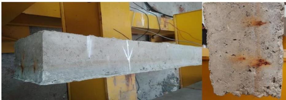
Fig 6 beam under acid attack
