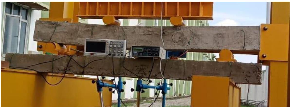
Fig 7 deflection of beam under acid attack
