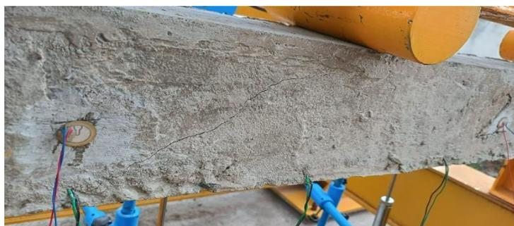
Fig. 4 Placing of transducer
