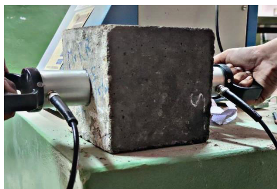
Fig 4: Ultra Sonic Pulse Velocity Test (UPV)
