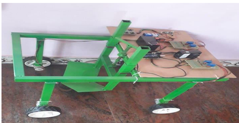
Figure.2 Working model of ginger harvesting machine
