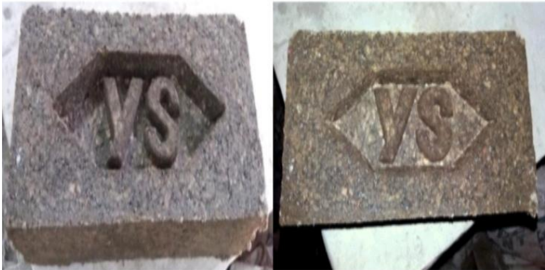
Picture: Papercrete Bricks After Casting
