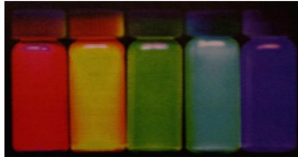
5 nm dots: red - 1.5 nm dots: violet(QDs prepared by colloidal synthesis)
