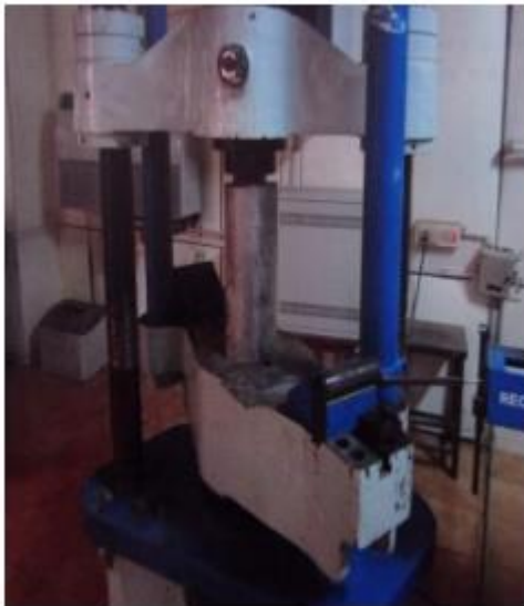
Fig 1 Testing of the Stainless Steel concrete specimen
