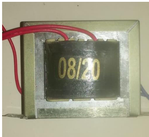
Figure.4 12-0-12 Step Down Transformer
