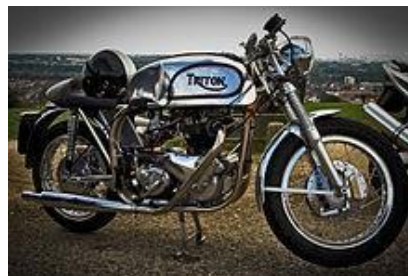
Fig 1.4: Norton Featherbed frame in a Triton.
