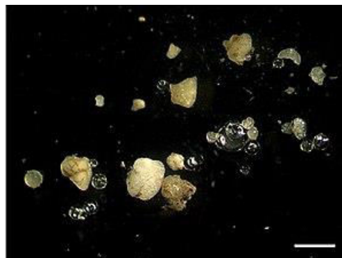
Microplastics among sand and glass spheres in sediment from the Rhine. The white bar represents 1 mm.
