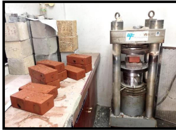
[Fig.3.4: Compressibility test]
