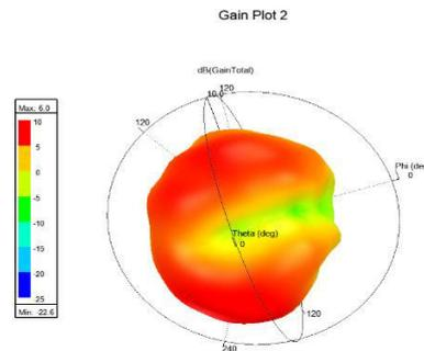
Fig. 3. 3D gain pattern of the proposed antenna.
