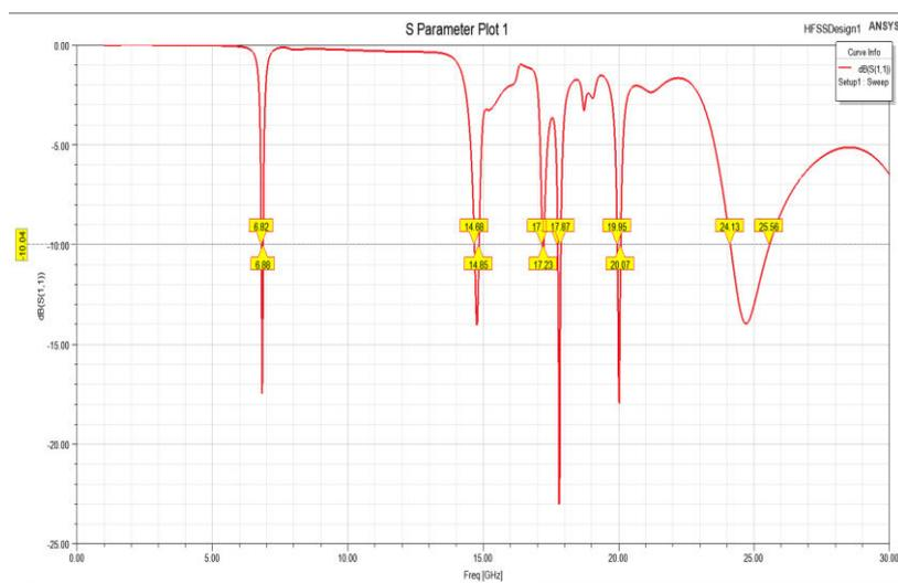
Fig. 2. Simulated return loss (S<sub>11</sub>).
