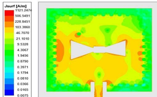
Fig. 5. Surface current distribution at 14.68 GHz.
