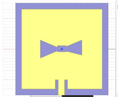
Fig. 1. Simulated SIW-based multiband antenna in HFSS.
