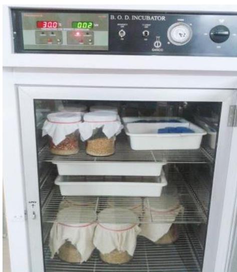
Figure 1: BOD incubator to study various levels of temperature & RH under laboratory condition
