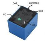
A 5V relay serves as an automated switch commonly found in control circuits to manage high-current devices with lowcurrent signals. The relay operates within a signal voltage range of 0 to 5V. The pin layout of the 5V relay is as follows:
