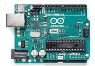
The Arduino Uno boasts 14 digital I/O pins, with 6 of them capable of PWM output, alongside 6 analog inputs. It features a 16 MHz ceramic resonator (CSTCE16M0V53-R0), USB connectivity, a power jack, an ICSP header, and a reset button. Fully equipped to facilitate your microcontroller projects, it offers seamless connectivity options—whether via USB to your computer or through power supplied by an AC-DC adapter or batteries. Its user-friendly design encourages experimentation
