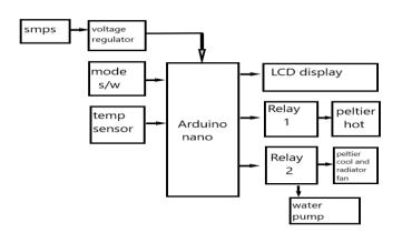
Smps is connected with voltage regulatorwhich controls voltage in Audrino Nano.
